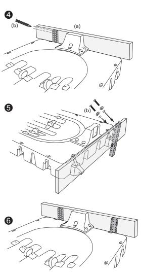
Note: If mounting port to wooden floating dock use 3/8" (9 mm) Lag Bolts (screw based)
